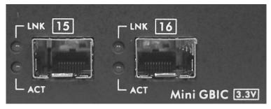
Figure 2-4. Combo SFP Slots port LED Indicators
